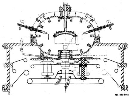
Fig. 3. Surface-conversion ion source and the 80 kV pre-accelerator under construction at LBL. In the magnetic bucket is a cylindrically-shaped converter which is focused at the entrance of a 4-section collimator shown adjacent to a high-perveance 3-electrode 80 keV pre-accelerator. The beginning of a TFF matching section is shown schematically.
