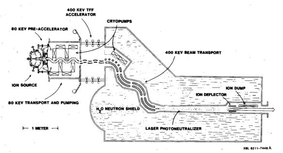
Fig. 2. Plan view of radiation-hardened 400-keY TFF-based beam line.
