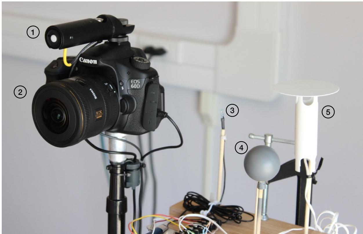
Figure 8.1 - Comfort sensing equipment: (1) Licor illuminance sensor for calibrating HDR images taken by (2) DSLR camera with 180° lens, (3) air velocity sensor, (4) mean radiant globe temperature sensor, and (5) shielded temperature sensor.
