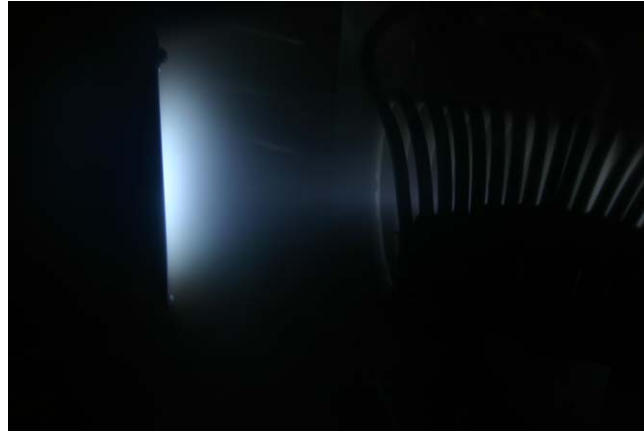
Figure 8. Open-shutter photograph through the vacuum window showing the enhanced optical emission when a surface (left) is hit by cathodic vacuum arc plasma (steaming from the right); for details see [107].
