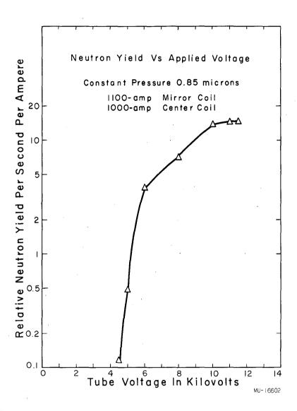
Fig 4. Neutron yield vs. applied voltage.
