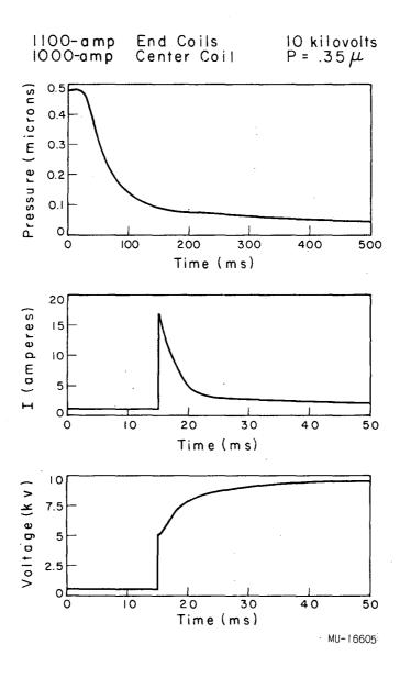
Fig. 3. Plots of pressure, current, and voltage vs. time for pulsed operation.
