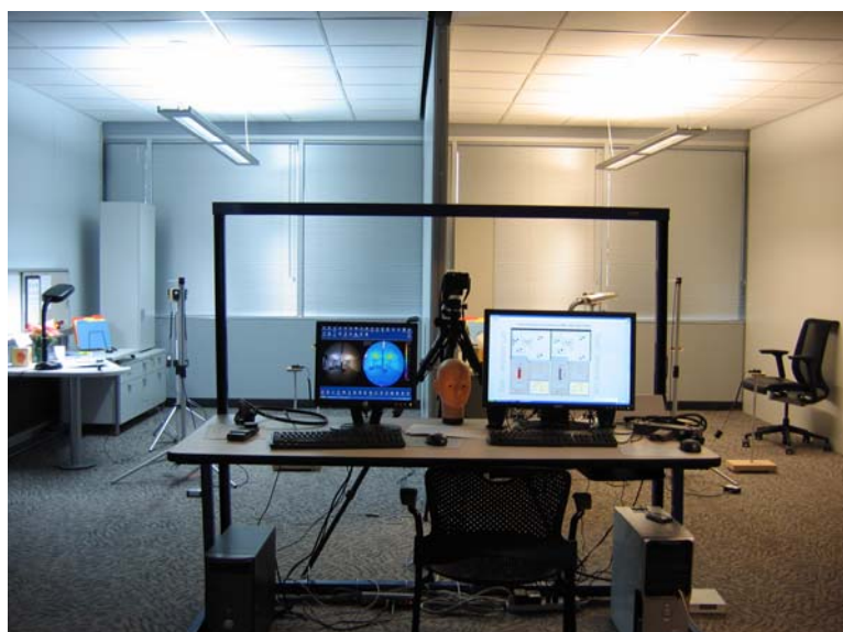
Figure 2: A scotopically-rich lighting system (left) is compared to a photopically-rich lighting system (right).
