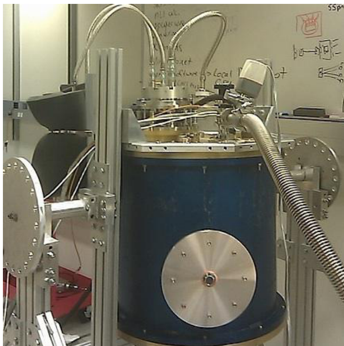
Figure 2.15: Outer shell of cryostat — Photograph of outside of cryostat.
