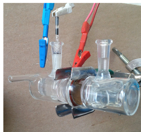
Figure 1. Photograph of the experimental setup. Red is attached to a working Pt foil electrode, blue is connected to a Pt mesh counter electrode against the back wall, and white is an Ag/AgCl reference electrode.
