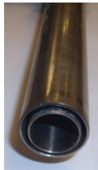
Figure 79: Close up view of the annular tubes used to pilot the flame.
