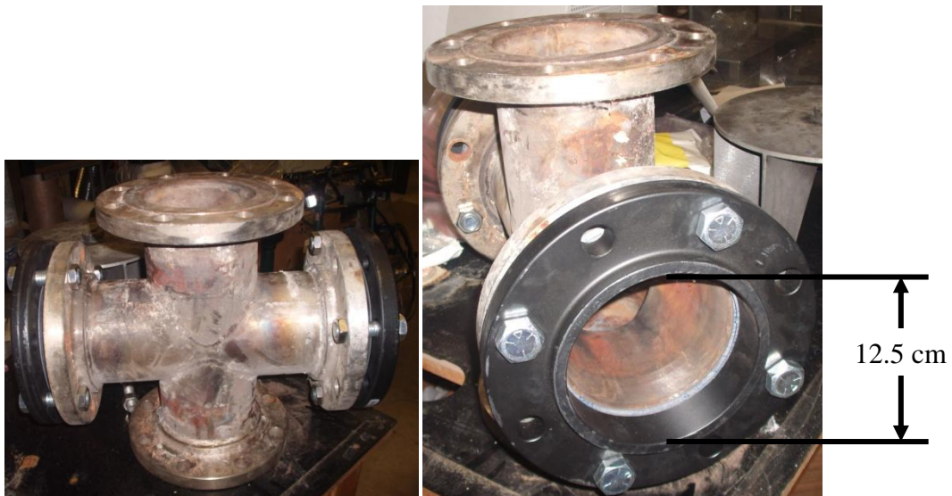
Figure 16: 12.5 cm cross around which the elevated pressure burner was designed.
