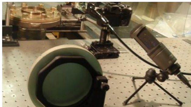
Figure 65: Atmospheric burner with microphone in place along with schlieren imaging system.
