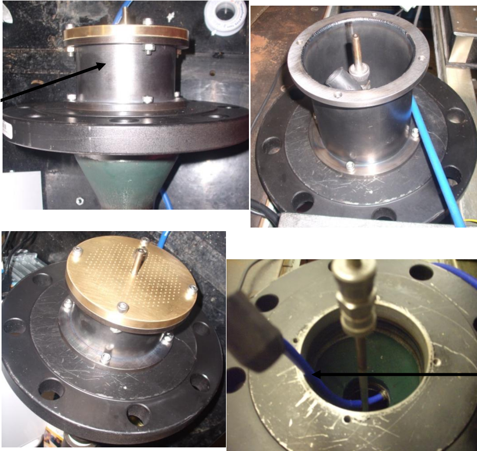
Figure 21: Elevated pressure VCB in various states of assembly.
