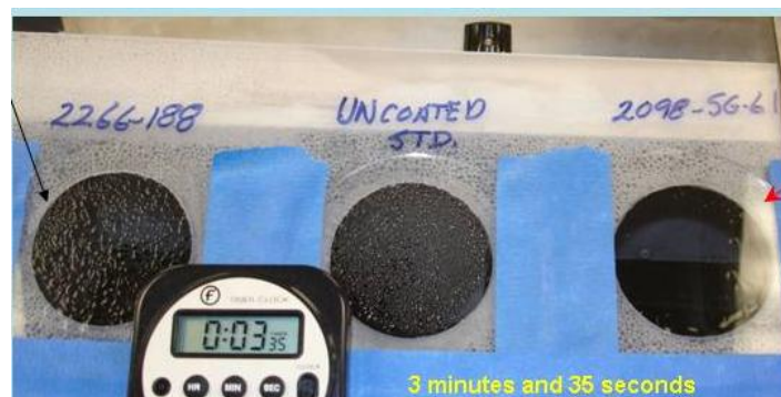
Figure 61: Example of the anti-fog performance of the coating from Hydromer, Inc. Image source: hydromer.com
