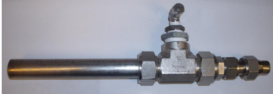
Figure 78: Primary components of the hydrogen piloted jet flame burner.
