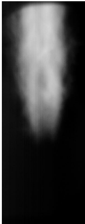
Figure 64: Direct image of a hydrogen lifted flame in the transient elevated pressure apparatus taken from video at 6000 fps.
