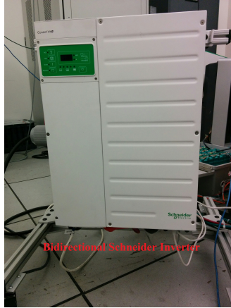
Figure 4.2: 6.8 kW bi-directional inverter (MBESS charger).
