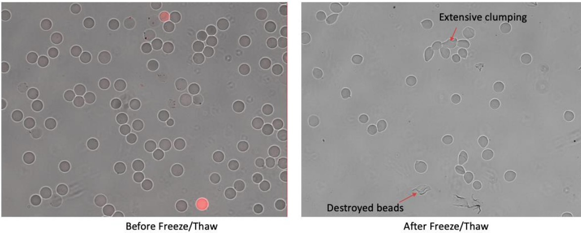
Figure 36: Gel bead destruction during the freeze/thawing process. Beads were stained with DAPI to identify beads containing single cells/nuclei
