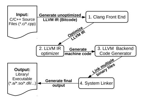
Figure 4.1: The standard LLVM compilation workflow for C/C++
