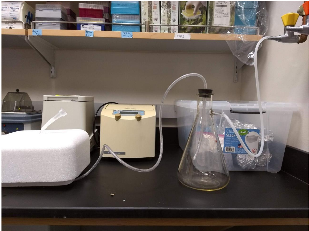
Figure S 3.1: Adapted vacuum pump in the pre-PCR room.
