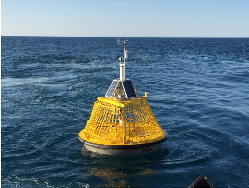
Figure 4.14: Waveheight measurement buoy located off the coast of Tillamook, OR. The pressure sensor gauge responsible for recording the wave height is attached to the buoy below. The buoy itself is responsible for the transmission of data. (N. N. D. B. Center, 2022)
