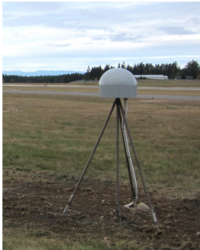
Figure 4.12: GNSS receiver with a sampling rate of one second stationed in Port Angeles, WA. (Team, 2013)
