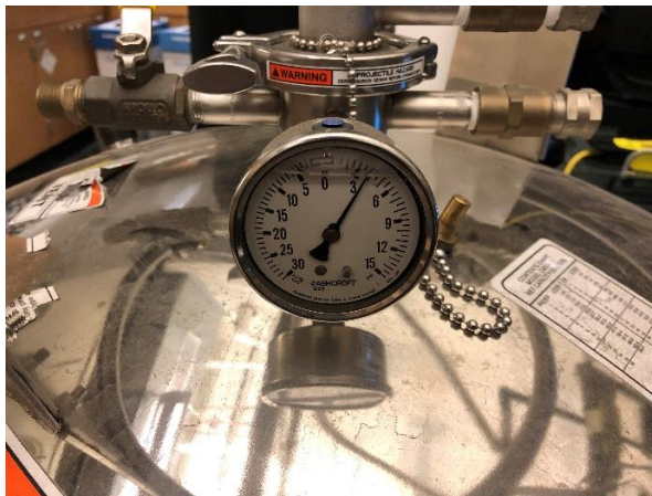
Figure 2.4.1. Images showing the connections between the Janis Research ST-300 cryostat and a liquid helium tank.
