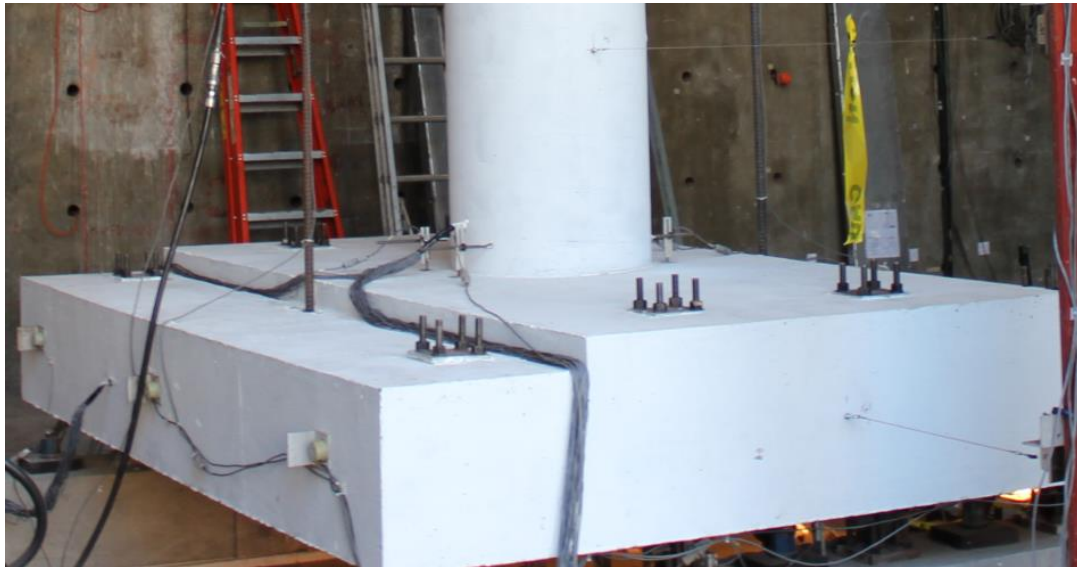
Figure 5.7 – Slab with drop cap in Specimen #3
