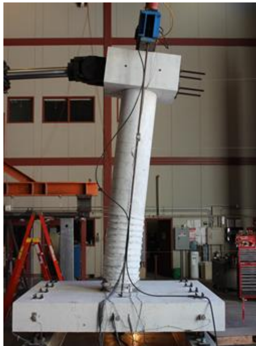
Figure 5.21 – Deflected shape of Specimen #1 at ductility 6
