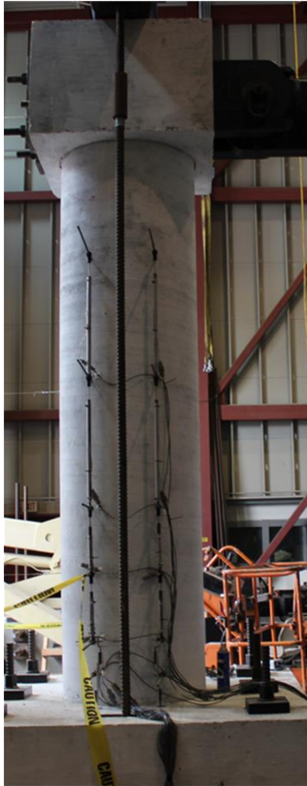
Figure 3.16 - Picture of displacement transducers mounted on west face of Specimen #1
