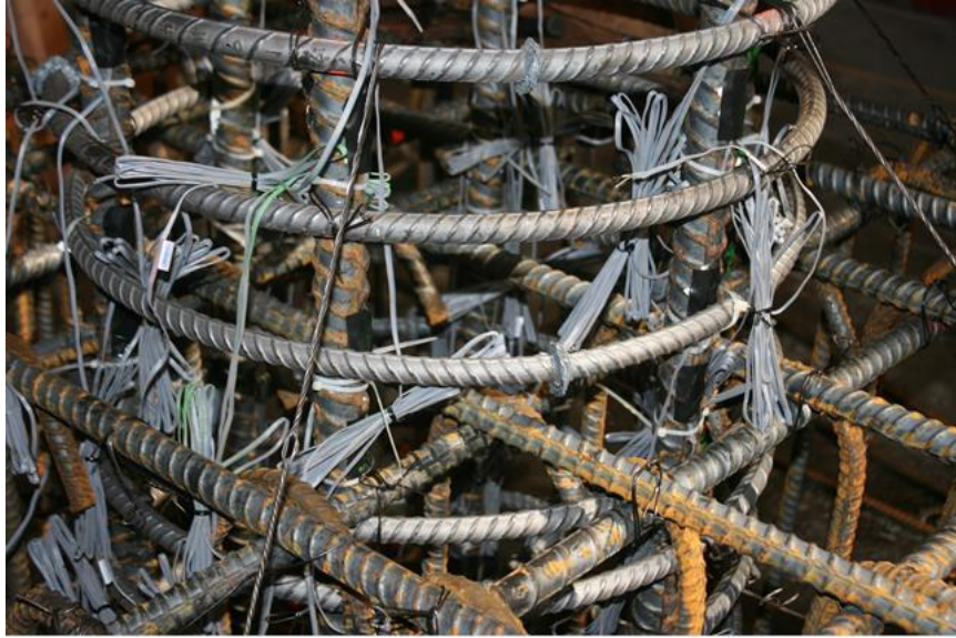
Figure 3.20 – Picture of strain gages on reinforcing bars of Specimen #1
