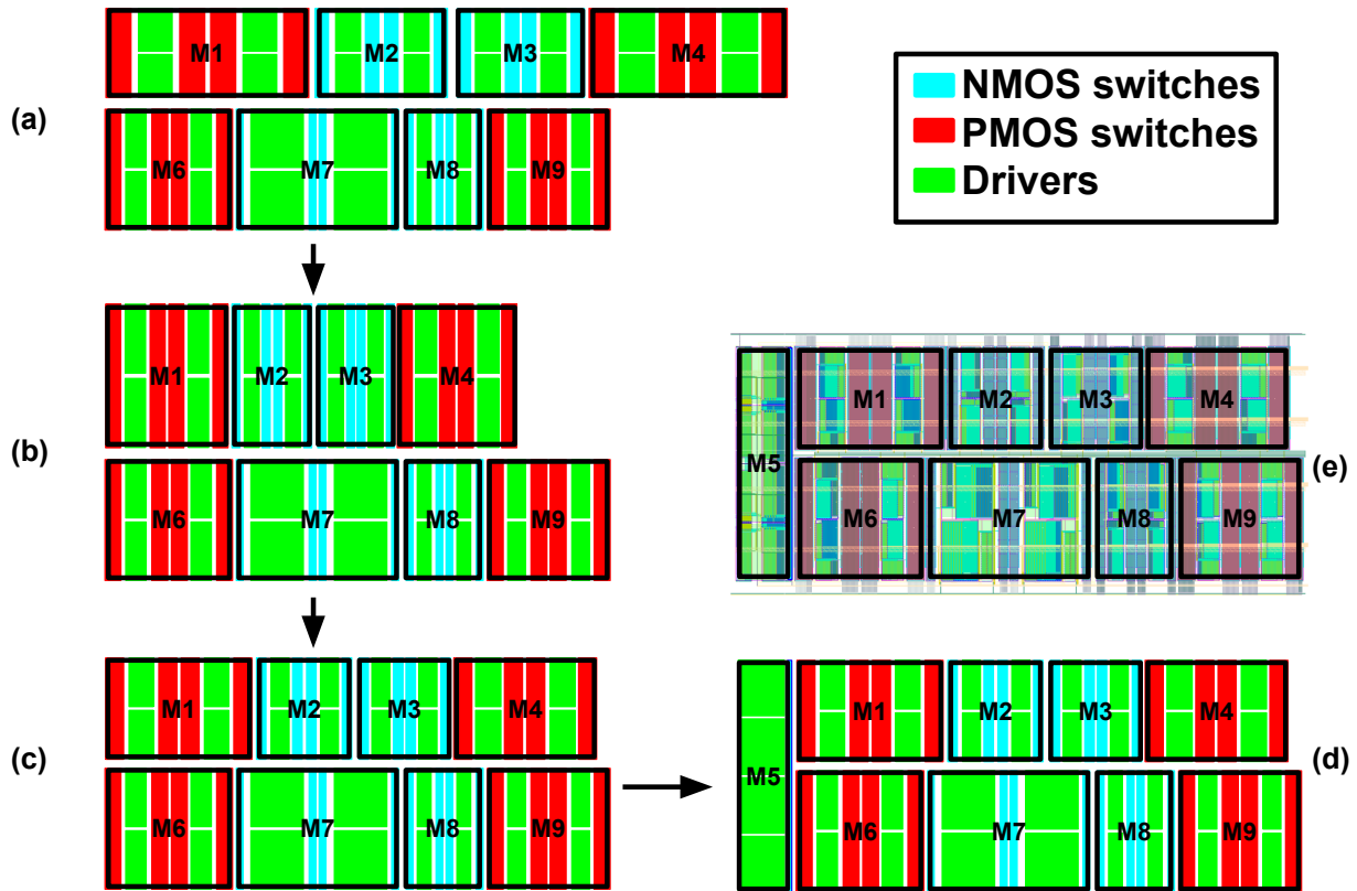
Figure 4.11: A binary search matches the width of the top row of power switches and drivers with the bottom row (a)-(c) before the final M5 switch is placed (d). The actual layout is overlaid by the cartoon in (e).
