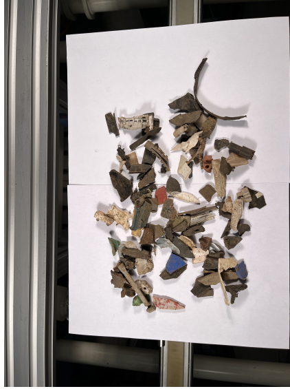
Figure 5.2: A controlled environment of various types of plastic on a sheet of white paper. The plastics have various colors and spectral signatures. © 2023 IEEE
