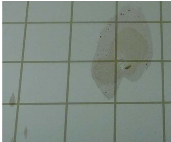
Figure 2.11. Picture of a cracked Ru film deposited on LTO after air exposure.
