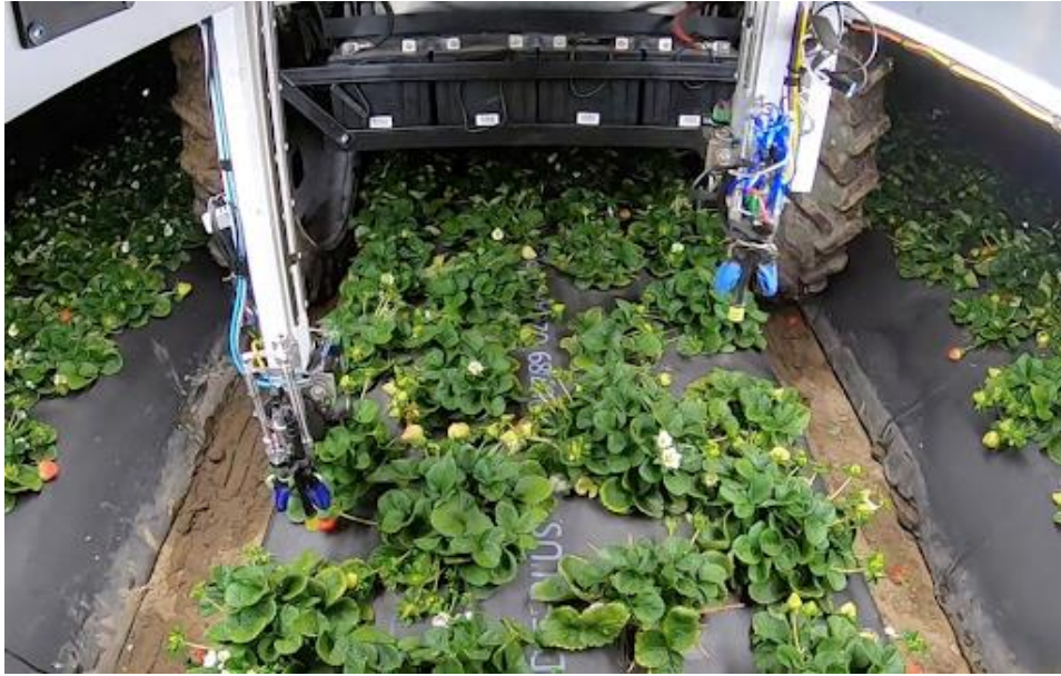
Figure 5: The interior of the mechanized harvester in operation, the blue claws and yellow suction cups are seen grasping at ripe strawberries.
