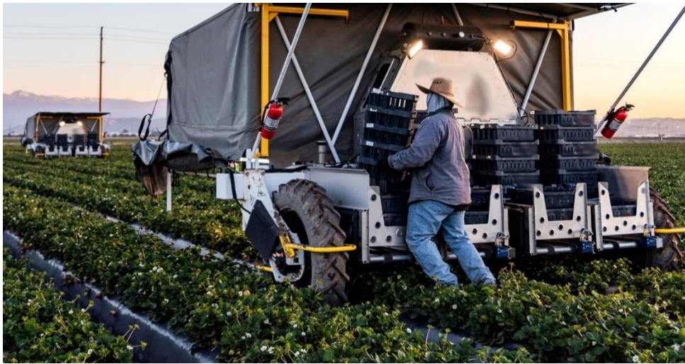
Figure 4: A single mechanized harvester moving through a strawberry field with the proprietary flats stacked on the back. A single operator can control eight of these machines at once.
