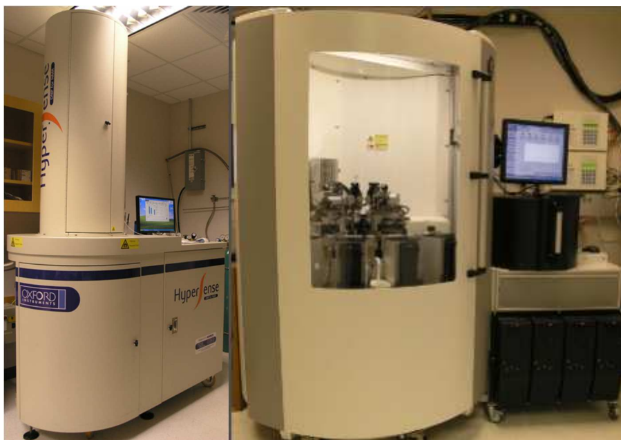
Figure 2.11: HyperSense (left) commercially available preclinical polarizer. 5T GE SPINlab (right) clinical polarizer for up to 4 sample vials in parallel with sterile fluid paths and a QC system for safe human injection. Standard operational steps of the HyperSense include: (1) the buffer is heated and pressurized, (2) the sample space is pressurized, (3) the sample is raised out of the liquid Helium, (4) the dissolution stick is lowered docking with the sample holder, (5) the solvent is injected dissolving the sample while preserving enhanced polarization.
