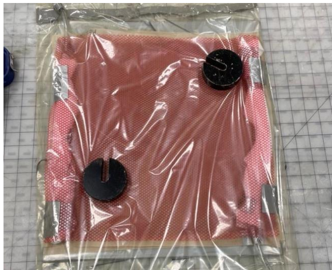
Figure 3: Initial VARTM bag setup and testing for leaks
