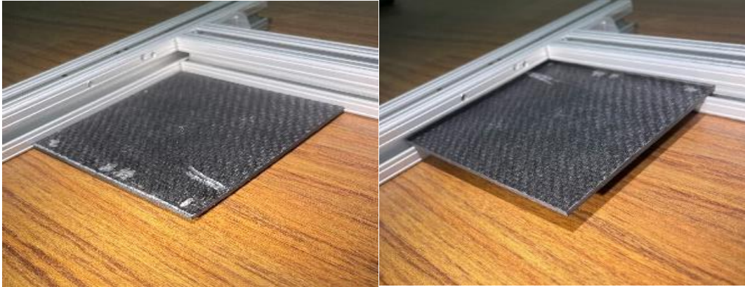
Figure 9: Capturing images with sample outside (right) and inside (left) the T slot fixture
