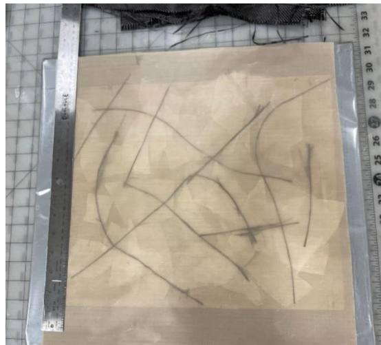
Figure 2: T300 fiber texturing during the preparation of the panel
