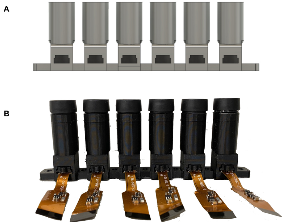
Figure 3.14: A. Shows the CAD rendering of our camera holder design and B. Shows the camera holders when printed with cameras inserted into them
