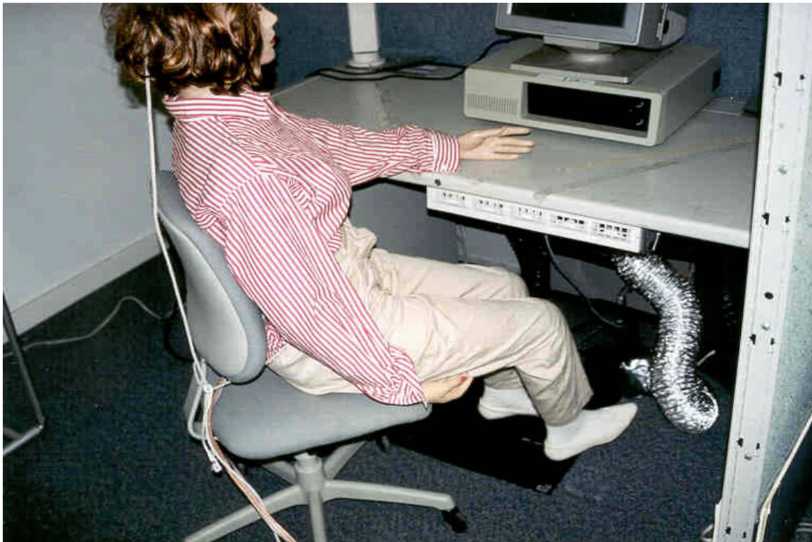
Figure 4. APACS unit mounted in test chamber with thermal manikin
