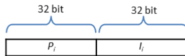
Figure 3.6. We reduced the matrix profile to 32 bits, then combined each matrix profile entry and its corresponding matrix profile index entry into a double-precision value to allow fast atomic updates.
