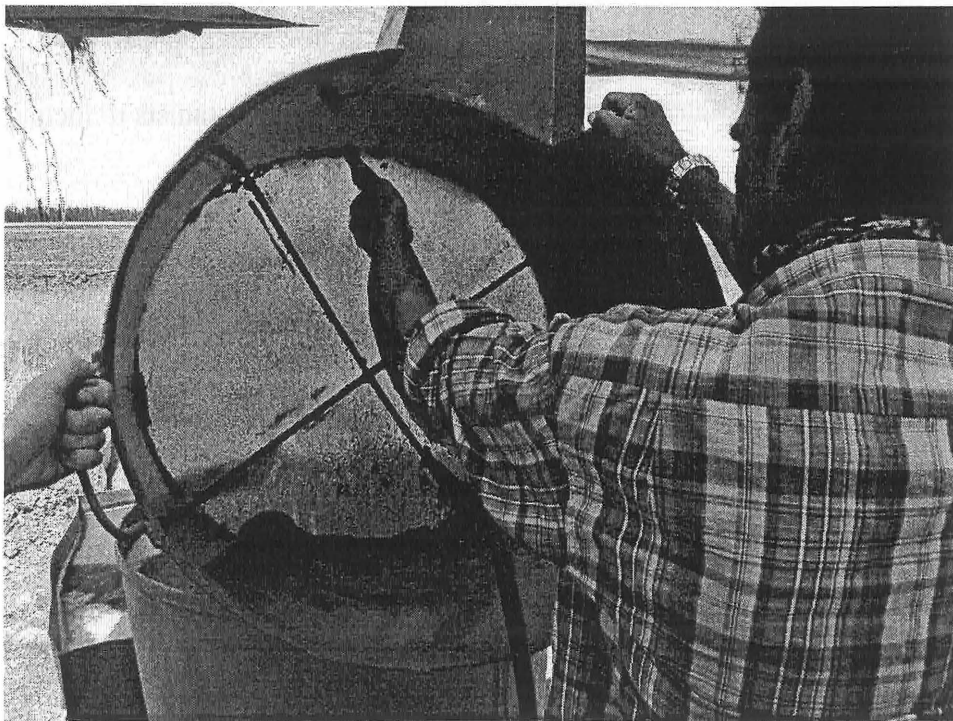
Figure 5: The 0.5 mm mesh used to capture the heavy residue
