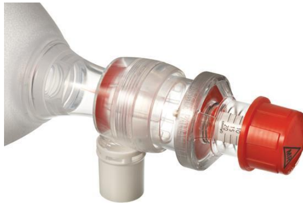
Figure 8: Ambu® PEEP disposable valve. This valve has a range of 1.5 - 20 cm H 2 O, maintained by the internal spring. [59]
