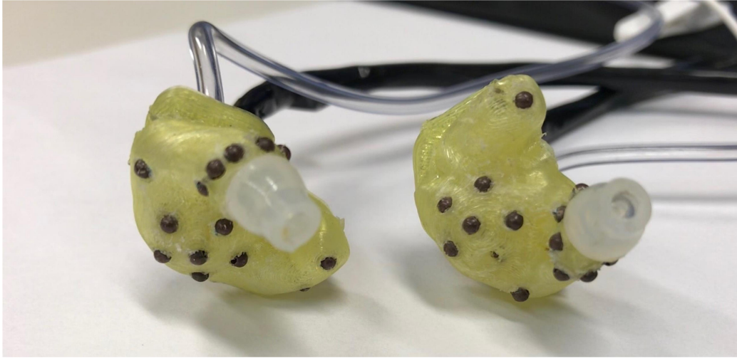
Figure 3.1: The earpieces fabricated from 3D CAD models of the subject's ear shown here embedded with 17 Ag-Ag/Cl electrodes each. A air tube comes through the lumen of the earpieces the provide sound directly the ear canal.
