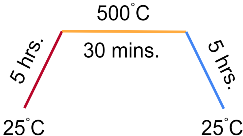
Figure 2.1. Heating Profile for tube furnace experiments for RE 3 Te 4
