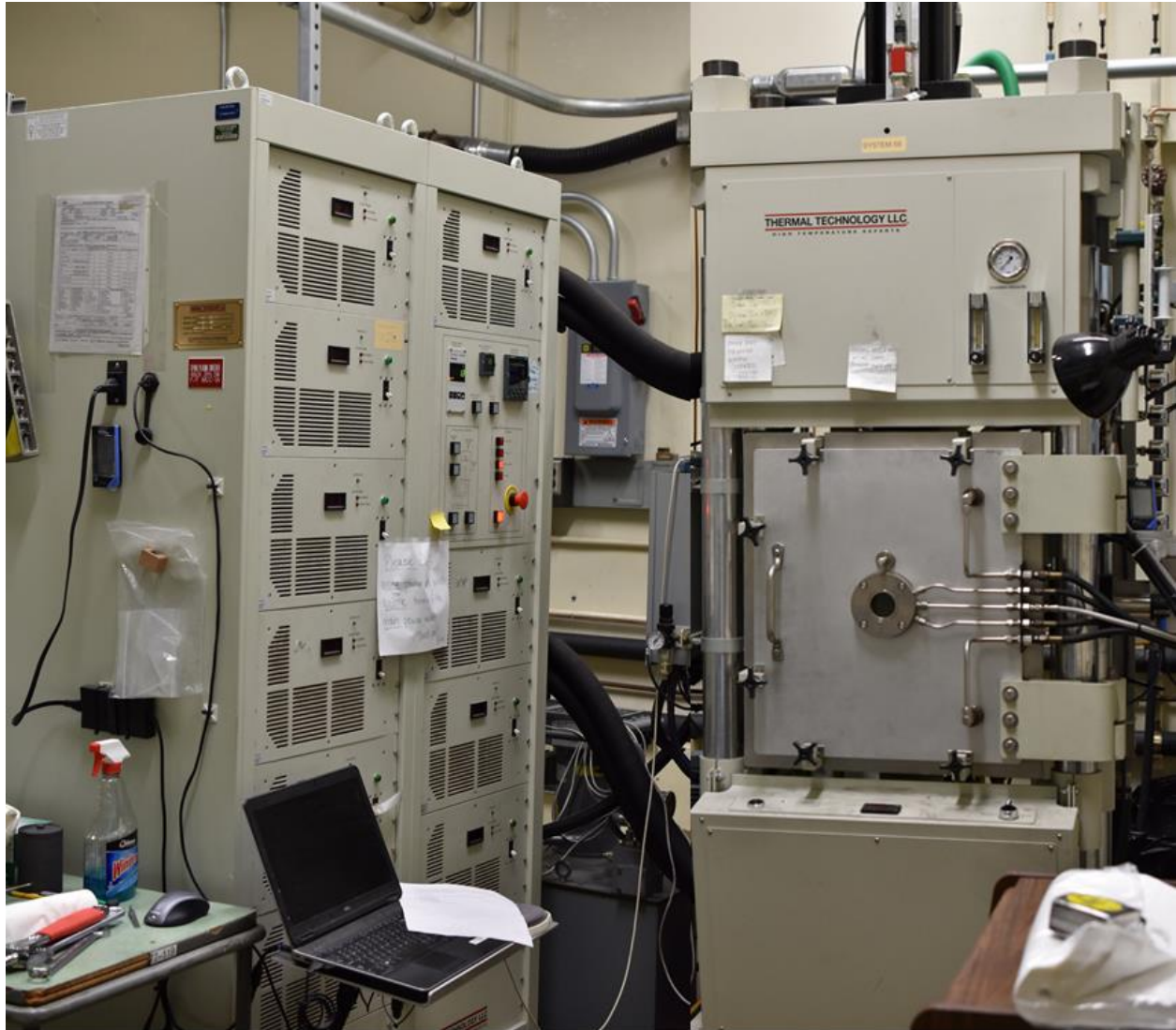
Figure 3.5. Thermal Technology LLC SPS 10-4 Advanced Technology furnace power supply (far left) and furnace pressing chamber (far right)
