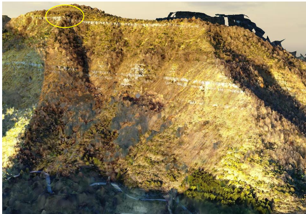
Figure 4.45. 3D SfM model of rockfall site near Cervaro village (Crognaleto). Primary rockfall source circled in yellow.
