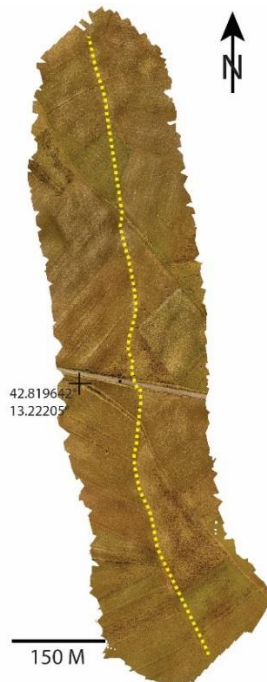
Figure 2.11. 3D digital terrain model from merged SfM and LiDAR data of the Piano Grande fault on the western toe of the Mt Vettore Massif. Approximate fault trace(s) indicated in yellow. Looking from the west. The left of the image is to the north. Mt. Vettore on the top of the image
