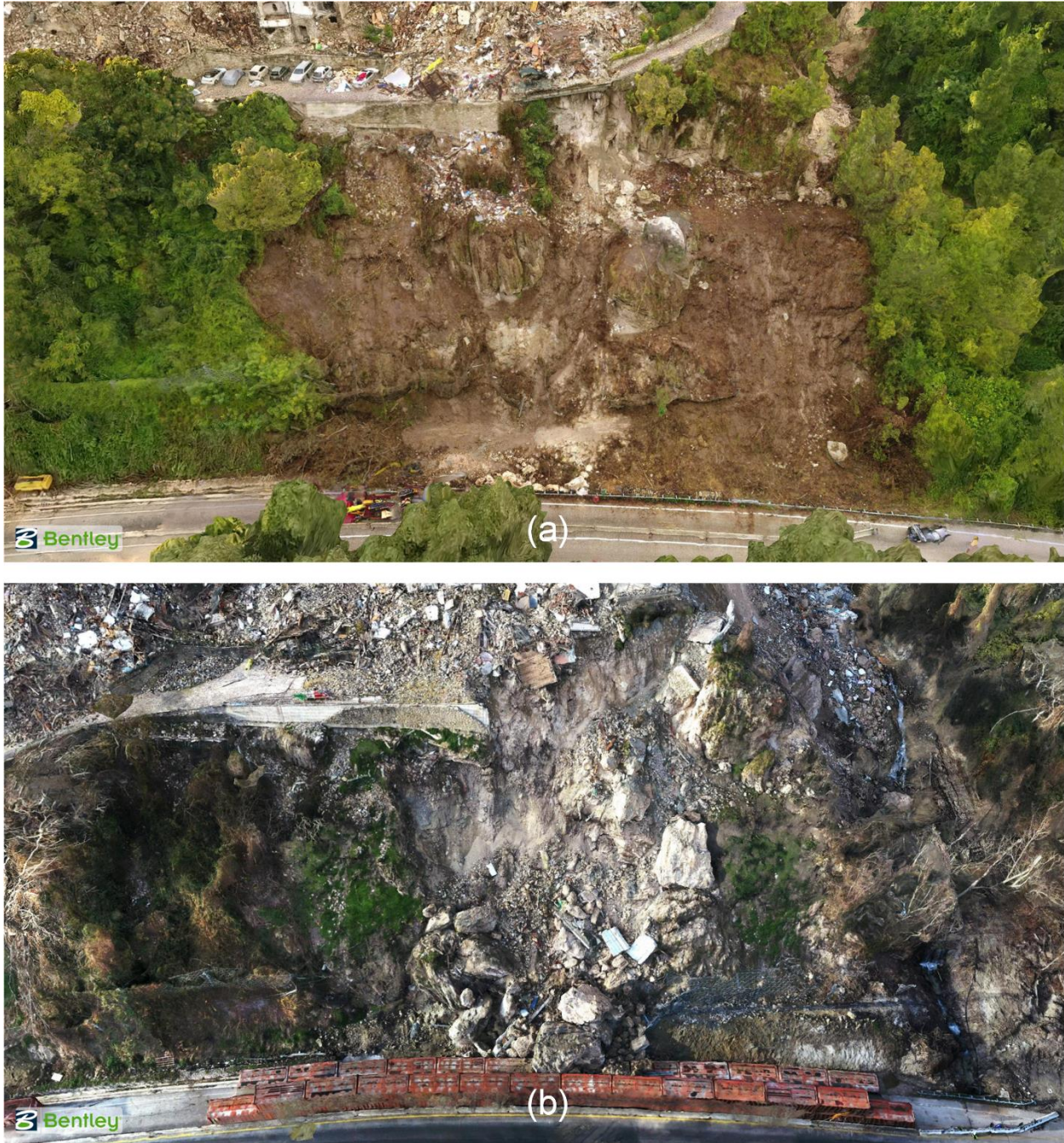
Figure 4.22. 3D model comparison of the landslide below Pescara del Tronto between September 2016 (a) and December 2016 (b).
