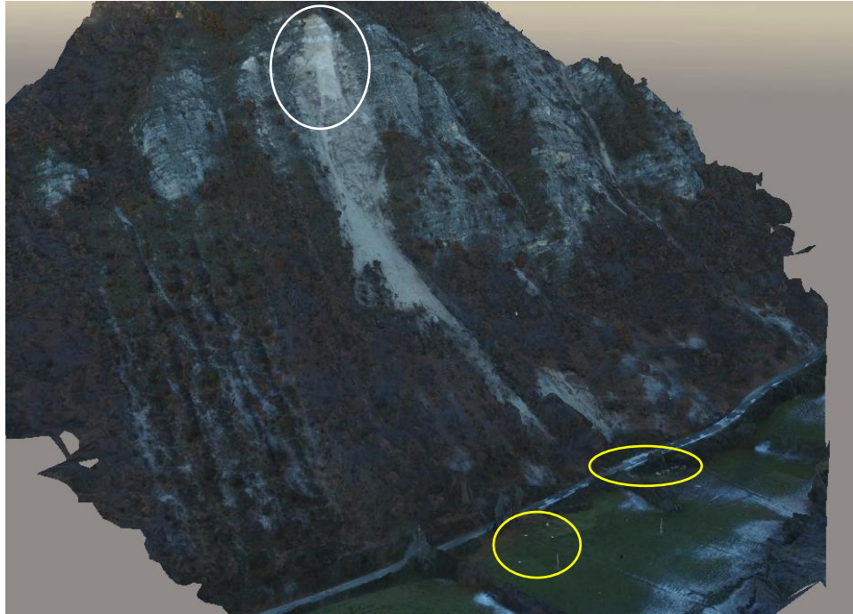
Figure 4.59. Pescia rockfall site 9b. 3D SfM model from UAV data. Boulders that have rolled into field below the road are circled in yellow. Source is indicated by white circle.
