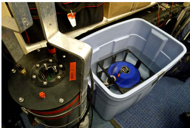
Fig. 1. Photograph of the acoustic decoy controller (left), mounted at the base of a spar buoy. The blue playback speaker is in the water on the right. (For interpretation of the references to colour in this figure legend, the reader is referred to the web version of this article.)
