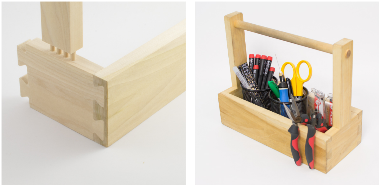
Figure 3.8: This poplar toolbox employs a variety of joints that would be difficult to create using current handheld and CNC tools.
