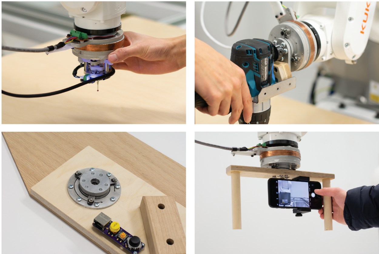
Figure 5.8: A. The probe uses the contact points of a kinematic coupling as electromechanical switches for detecting when the probe tip has been displaced. B. The drill is mounted to the bracket using the fasteners that secure the drill’s gearbox to its body. C. The track is attached to the robot through a flexure, which is designed to compliant out of the plane, but rigid within the plane. D. The camera uses an off the shelf smartphone mount.
