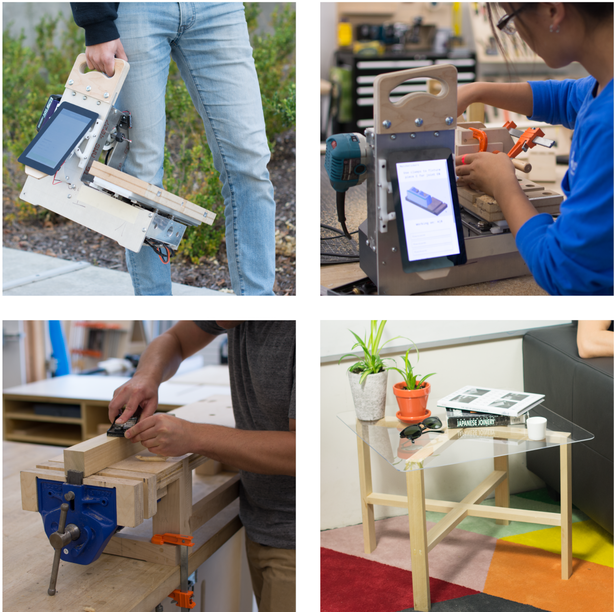
Figure 3.1: (Top Left) MatchSticks is a digital fabrication system for woodworking. (Bottom Row) Wooden objects larger than the size of the machine can be fabricated using a parametric joint library. (Top Right) We evaluate our system with users who followed an on-screen tutorial to create a parametric box.
