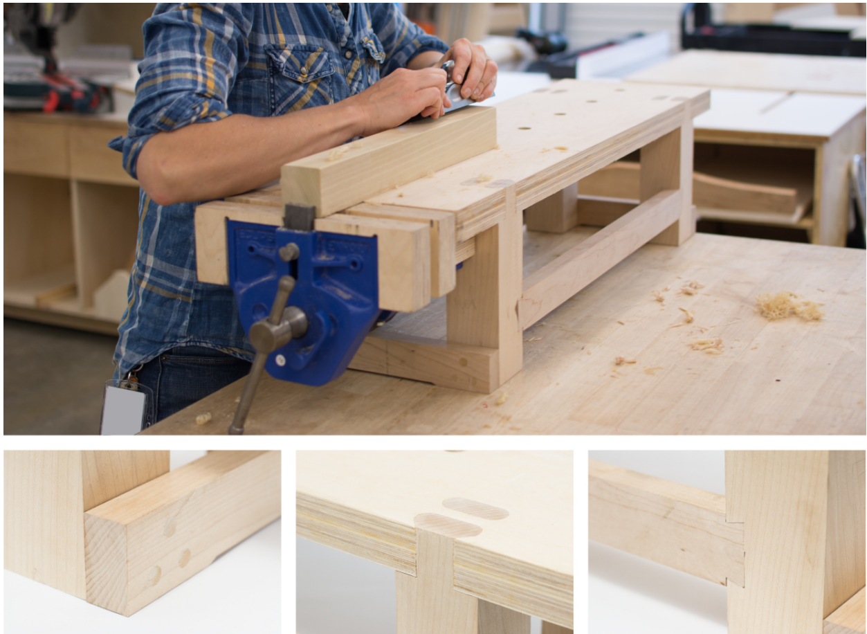
Figure 3.11: This miniature workbench highlights complementary capabilities of traditional CNC routers and MatchSticks .
