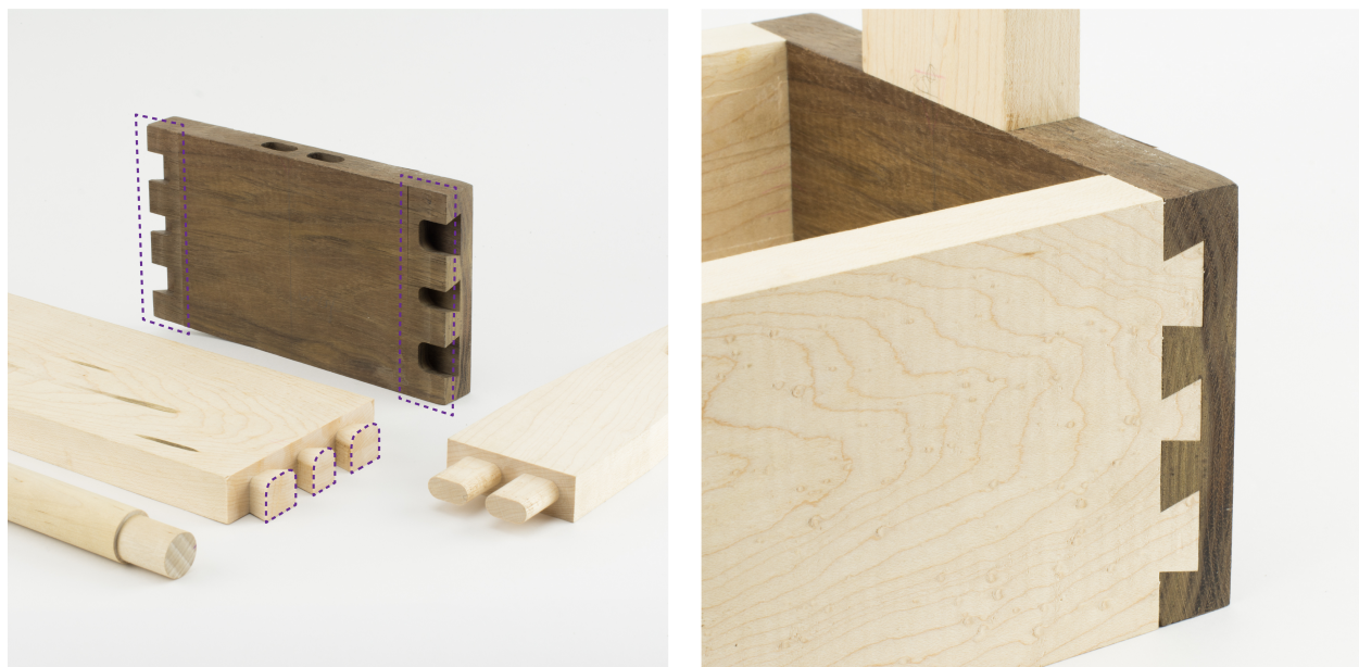
Figure 3.9: A variety of specialized router tools exist in woodworking. This example was created with a tapered router bit. The joints are highlighted by the alternating use of Peruvian Walnut and Birdseye Maple. While the boards used to construct this box have not been planed flat, the joints fit snugly because the contact areas of the joint have been locally planed (Left, locally planed area outlined).
