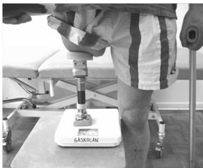
Fig. 3 ▲ Transfemoral patient with short prosthesis for axial loading
