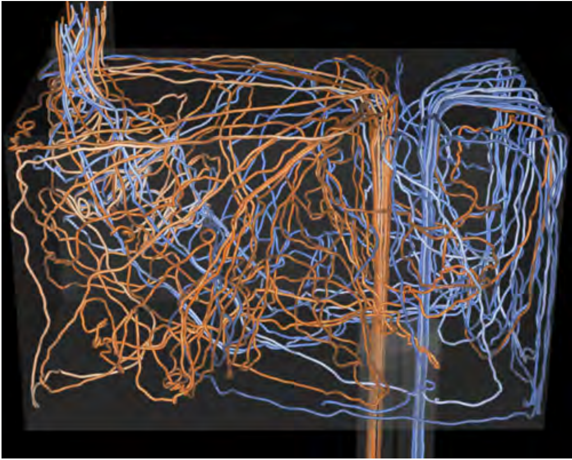
Figure 7: Integral curve computation lies at the heart of visualization techniques like streamlines, which are very useful for seeing and understanding complex flow-based phenomena. This image shows an example from computational thermal hydraulics. Algorithmic performance is a function of many factors, including the characteristics of the flow field in the underlying data set. Image courtesy of Hank Childs and David Camp (LBNL).
