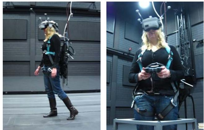
Figure 2: The virtual reality setup. The left image depicts a participant walking on the omnidirectional treadmill during the learning phase. The right image shows a participant pointing to a target during the testing phase by facing the target and pressing a button on a gamepad.
