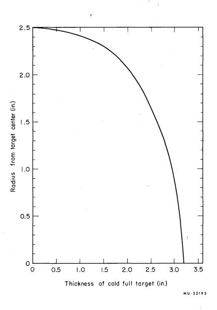
Fig. 7. A plot of the thickness of the cold full target as a function of the distance from the beam axis.
