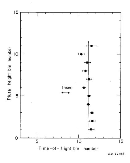
Fig. 17. Plot of the position of the Gaussian fitted to the hydrogen data as a function of pulse-height bin. It appears to be consistent with the straight line drawn through the data.
