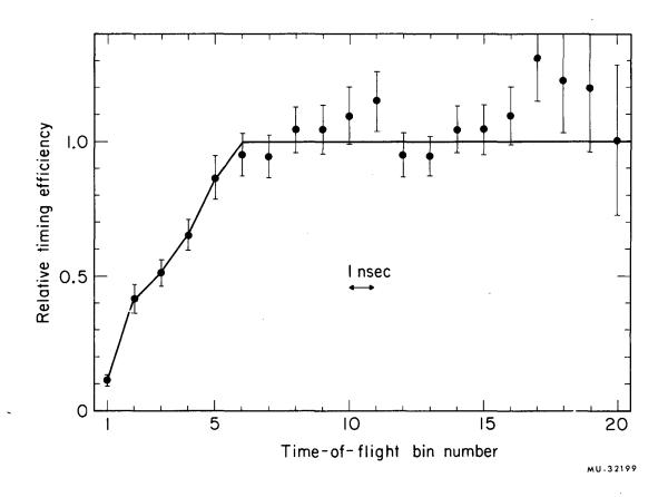
Fig. 13. Plot of the relative timing efficiency as a function of time-of-flight timing on the film for running condition GDB.
