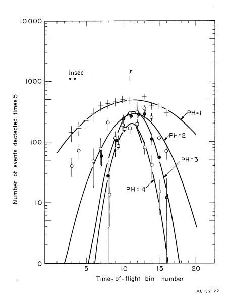
Fig. 15. Time-of-flight distribution for detected particles for 50-MeV pions on hydrogen (GDN) for various pulseheight bins. Where data points overlap the higher pulseheight bin is displaced to the right. The curves are single Gaussians fitted to the data. The data have been multiplied by five to correspond to similar numbers of incident pions, as in the deuterium case.
