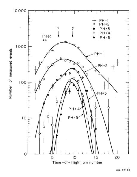
Fig. 14. Time-of-flight distributions of detected particles for 50-MeV pions on deuterium (GDN) for various pulseheight bins. The curves are the fitted Gaussians. Their center positions are indicated. Note the preponderance of neutrons at low pulse heights and their absence at high pulse heights.
