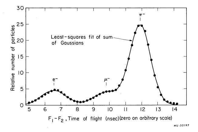
Fig. 4. A typical time-of-flight distribution for beam particles between  $F_1$  and  $F_2$  used to determine the beam composition. The position of the three distributions is indicated and a leastsquares fit of three Gaussians drawn through the data. This fit indicates 70.6% of the beam is  $\pi^-$ , 13.9% of the beam is  $\mu^-$ , and 15.5% of the beam is  $e^-$ .
