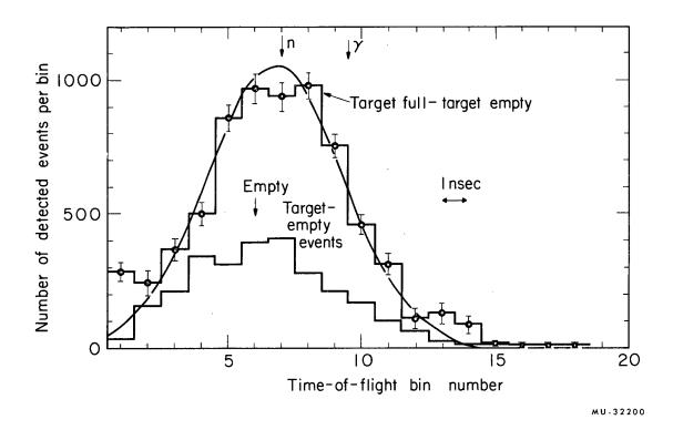
Fig. 19. The time-of-flight distribution of detected particles in the lowest pulse-height bin plotted for stopping pions in deuterium (GDN). The target-empty events are indicated and have been shown for comparable numbers of incident particles. The curve is a two-Gaussian fit. Arrows indicate central positions of timing distributions.
