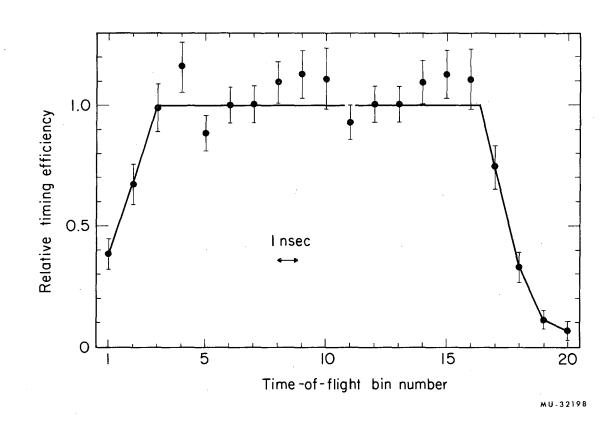
Fig. 12. Plot of the relative timing efficiency as a function of the time-of-flight timing on the film for running condition GDN.
