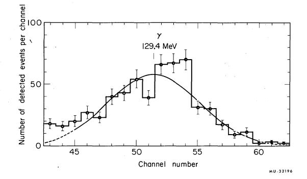
Fig. 21. Plot of the radiative-capture photon energy distribution in hydrogen as a function of channel number in the pulse-height analyzer used. The Gaussian fit to this distribution shows the energy resolution of the system to be  $(8.6\pm0.6)\%$  half width at half maximum.
