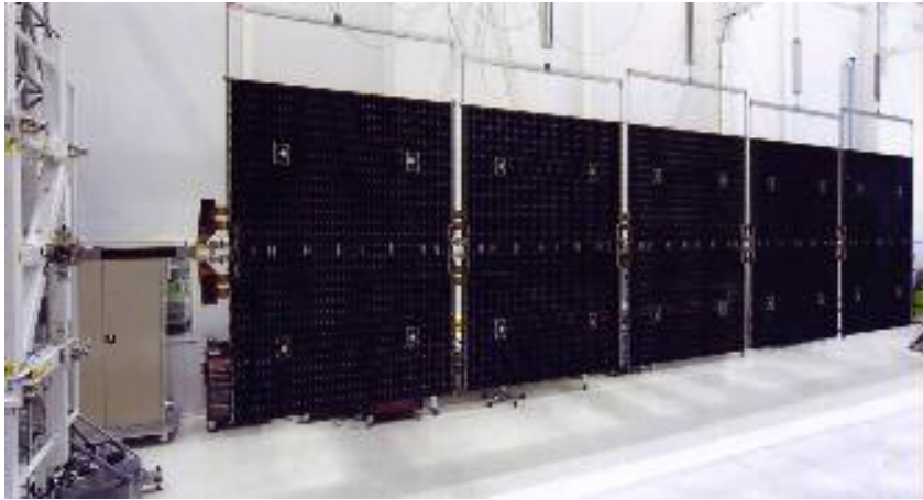
Fig. 5 One wing of Dawn's solar array extended on the deployment rig
