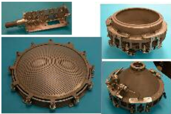
Fig. 6 Ion thruster components; clockwise from top left neutralizer, plasma shield views from top and bottom, and the iron grid
