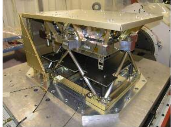
Fig. 2 The visible and infrared spectrometer (VIR) mounted to the vibration test table with GSE fixturing
