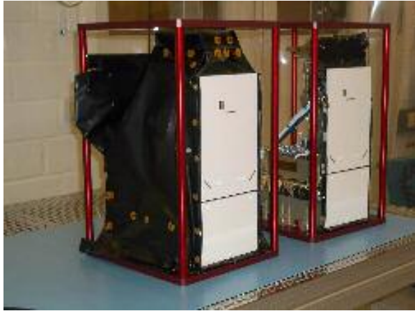
Fig. 1 Two assembled framing cameras, covered by thermal blankets, after successfully completing environmental testing
