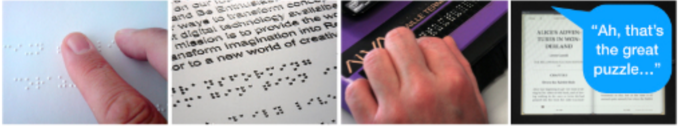
Figure 3.1: Examples of how PWVI might read a book. From left to right: (a) Traditional Braille books are written as raised characters on high-quality paper, (b) Twin-vision books are written in both print and Braille, which, here, appears beneath the printed text, (c) Refreshable Braille displays dynamically raise Braille characters to display digital text, and (d) Text-to-audio technologies, like audiobooks, or e-books read by the iOS native screen-reader VoiceOver, can be used to vocalize digital texts. 1
