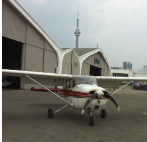
Figure 1.3: Cessna 172 two-blade propeller with severe rolling-shutter distortion. This photo was taken by Laura Waller using an iPhone camera [182].
