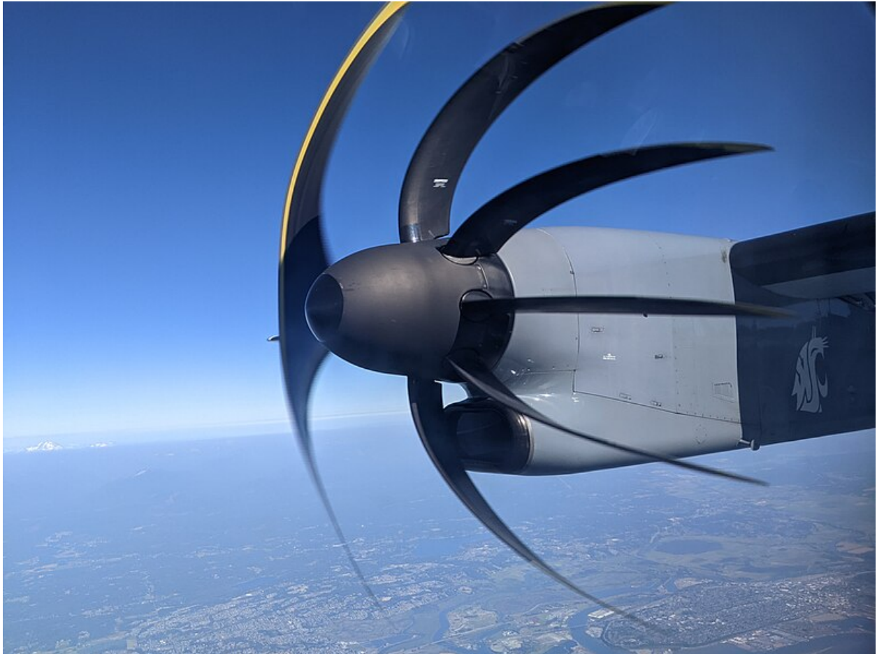
Figure 1.2: A de Havilland Canada Dash 8 Q-400 six-blade propeller with severe rolling-shutter distortion. This photo was taken by Richard F. Lyon using a Google Pixel 3 camera [50].
