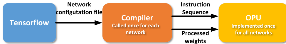
Figure 4.1: OPU working flow.
