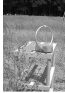
Figure 2. HFI transmitting and receiving antennas: (a) Loop transmitter and related power supply; (b) Electric field sensor with a long supporting beam and a big base plate; (c) Magnetic field sensor.
