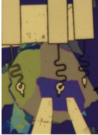
Figure 2.11: hBN-encapsulated graphene device with transferred scanning top gate serpentine electrode, donut inner diameter is 3 \mu\text{m} .
