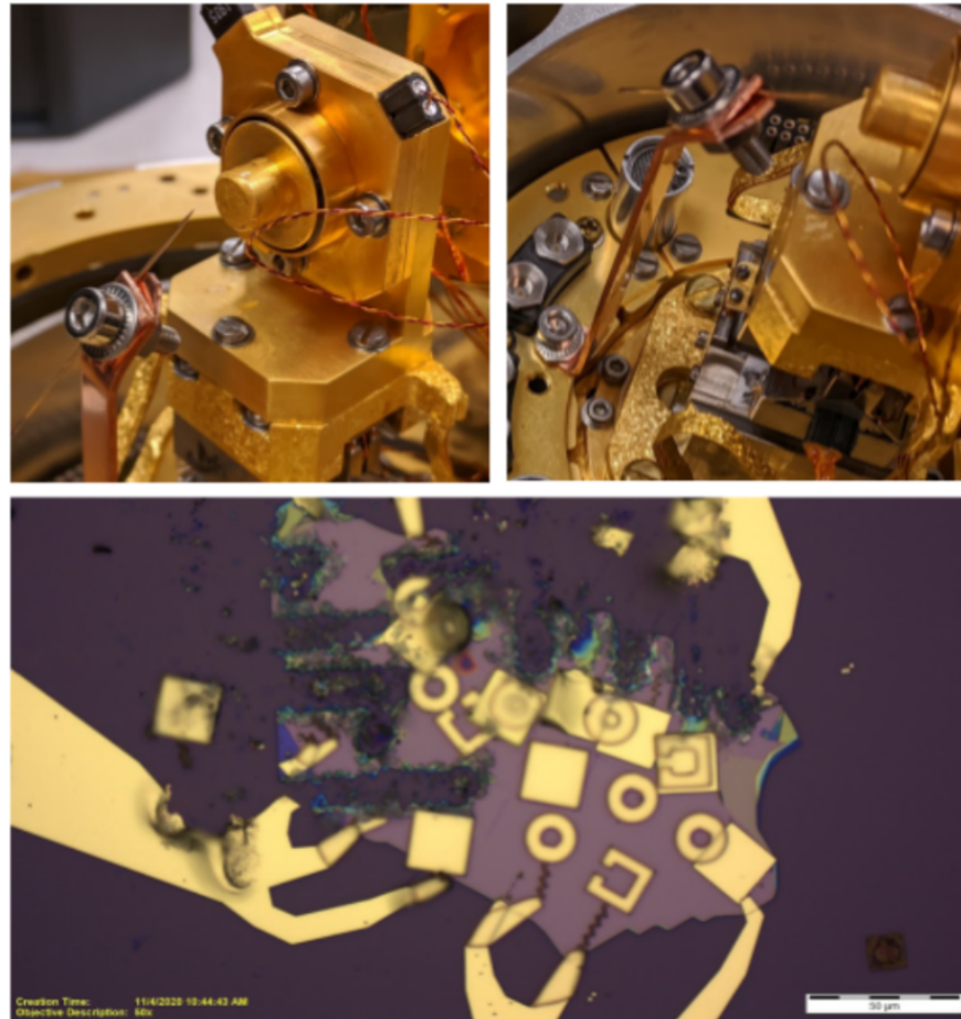
Figure 3.16: Montana crude probe tip manipulation setup and damaged sample
