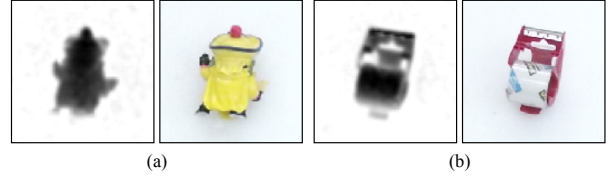
Figure 2.7: Two failure modes of CGPN. (a) shows the unmodeled sim-to-real gap on the object’s surface, and (b) shows the limitation of the depth image in representing 6-DoF grasps.
