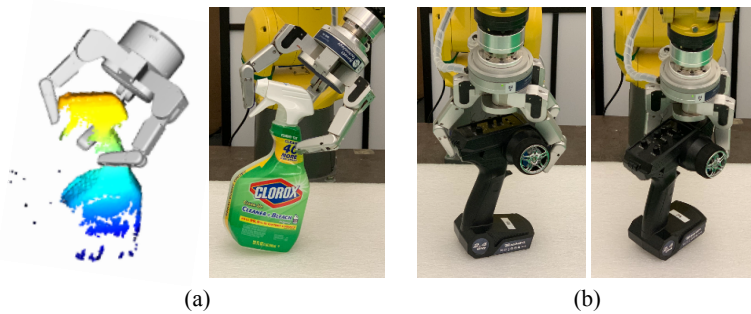
Figure 4.9: Two failure modes of MF-GPD. (a) shows the object slippage due to lack of contact detection with incomplete point clouds, and (b) shows the net object movement when unbalanced forces are applied.
