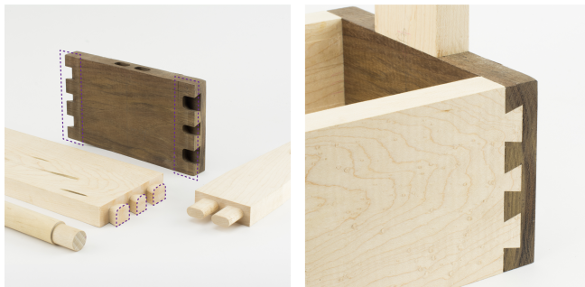
Figure 10. A variety of specialized router tools exist in woodworking. This example was created with a tapered router bit. The joints are highlighted by the alternating use of Peruvian Walnut and Birdseye Maple. While the boards used to construct this box have not been planed flat, the joints fit snugly because the contact areas of the joint have been locally planed (Left, locally planed area outlined).
