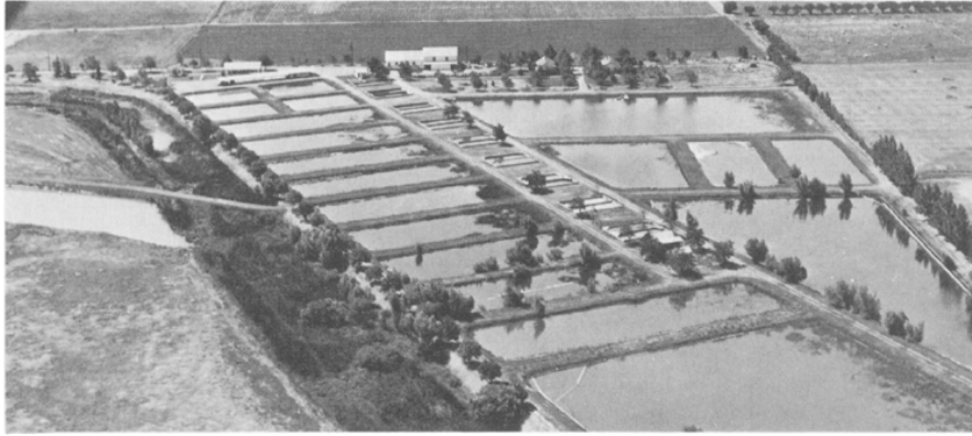
FIGURE 38. Central Valleys Hatchery. Warmwater fish rearing ponds on left, concrete daphnia tanks in center aisle, and broodstock holding ponds on right.
