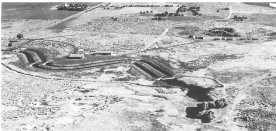
FIGURE 51. Aerial view of Fish Springs Hatchery shortly after completion in 1952, showing spring area with six earthfill ponds in foreground, food storage and utility buildings left center, and employees' houses on right.
