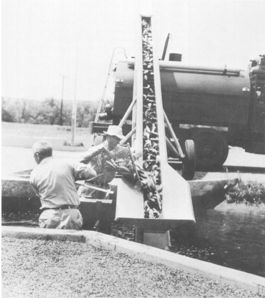
FIGURE 46. Loading trout for planting with a mechanical fish loader, San Joaquin Hatchery. Photograph by William M. Carah, May 1956.
