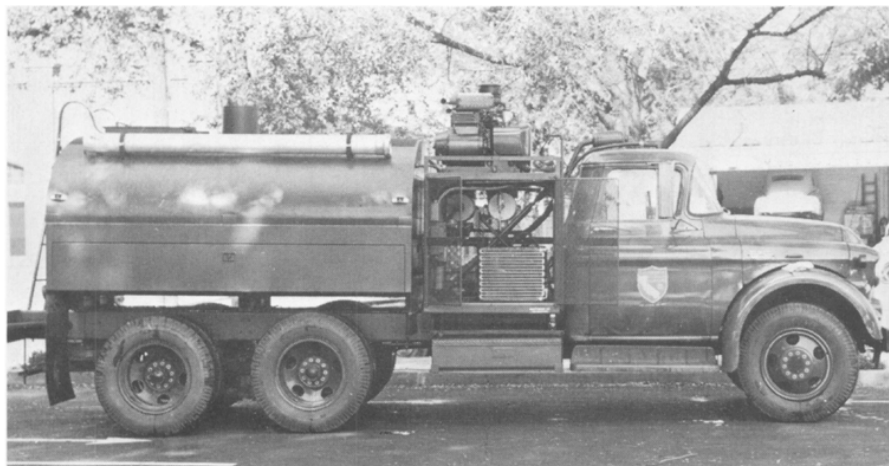
FIGURE 31. 1961 model fish hauling truck; 2,000-gallon water capacity; V-6 engine under the hood; carrying capacity 3,000 pounds of 6- to 10-inch trout. Gasoline powered generators develop power for operating water circulating pumps and refrigeration units. Aeration of water is by a combination of venturi aspirator and overhead spray. Photograph by Bert Williams.
