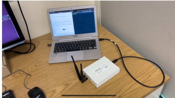
(b) The B210 plugged into the laptop via USB
