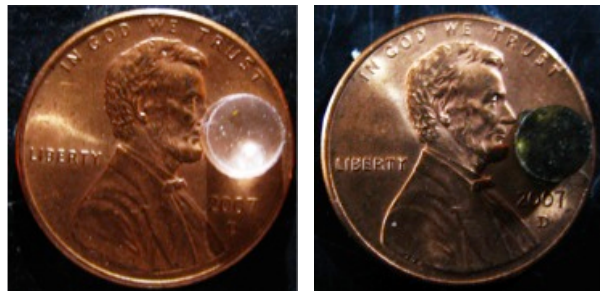
Figure 8. PDMS disks (5 x 2 mm). Left: blank disk. Right: disk loaded with UNCPs and RBS. Pictured with a US 1 cent coin to indicate relative size.
