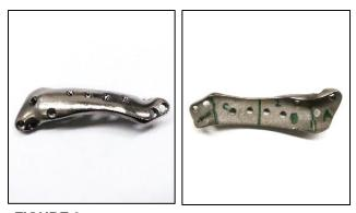
**FIGURE 3:** Additively manufactured Ti 6AL4V bone plate to correct radial deformity. The finished top surface (left) and the unfinished bottom surface (right) are shown.
