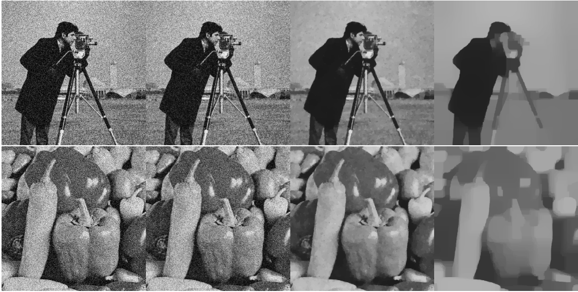
Figure 2.1: Sample images along the solution path of the search heuristic. Images are arranged from left to right as follows: noisy input, first candidate image (50% reduction of total variation), best candidate by MSE, and candidate generated after the optimal image.
