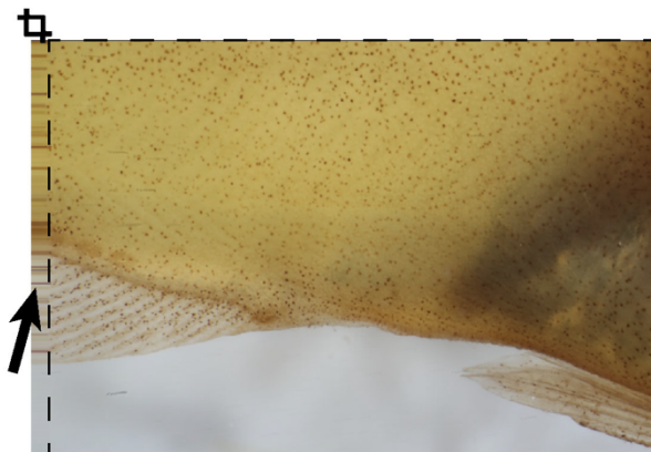
Figure 4. Example of artifacts created during focal stacking. Artifacts such as blurred areas along the edge of the Z-stack may appear (black arrow) and should be cropped out of the image.
