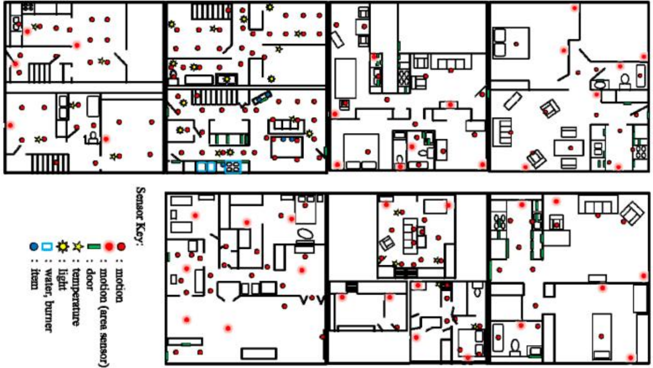
Figure 6.16: Sensor layout for the seven CASAS smart environment testbeds[84] energy optimization algorithms. Processing energy cost represents a small portion of the whole IoT system energy consumption. However, we found that if we reduce the processing energy cost, we reduce the underlying costs (transmission and sensing). As an example, in our comparison of fall detection approaches, table 6.14, one of the most complex approaches in computation is video processing, which is also costly in transmission and sensing.
